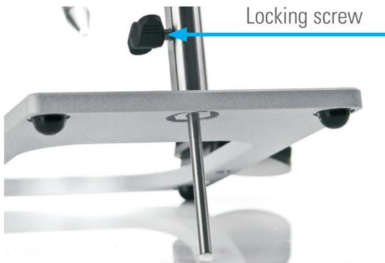
You also have the option of changing the angle of inclination for the microscope. To do so, undo the locking screw in the stand. A metal support now extends and forms an additional stand leg. Move the microscope into the desired position and tighten the screw again.
