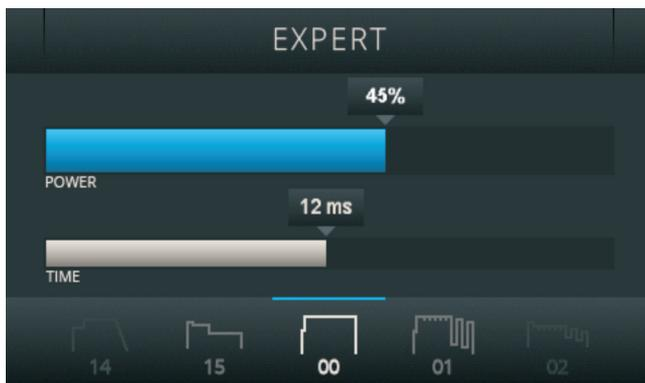
The expert menu can be activated in the settings user level. After activation, the expert menu appears as a separate user level, which can be accessed by pressing and holding the multifunctional controller. The various welding characteristic curves are stored in the expert menu, which have been developed and defined in the start menu for the preconfigured metals and welding geometries. However, here they are shown without content-related assignment. This mode is designed
