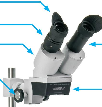
Look through the two oculars (1) and move the ocular tubes (5) inwards or outwards by moving the prism housing (3) in or out. The interocular distance is correct if the range of vision as viewed through the two oculars is complete and is united as a single complete image. The interocular distance should be individually set for each user. A spacer sleeve ensures the correct distance for focussing.
