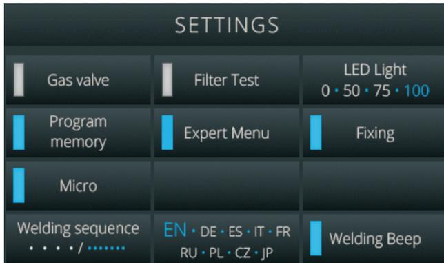
In the "settings" user level, it is possible to implement basic settings and perform various test functions. The activated settings are shown in blue.
