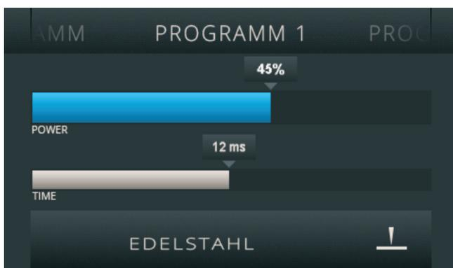
Pressing and holding the metal selection in the start menu or the welding curve in the expert menu results in the current parameters set being accepted in the program memory menu. 20 storage spaces are available here for individual storage. In the first step, the program space is selected by swiping to the left or right. The set data is then accepted by pressing the "continue" button. Saved data cannot be deleted. It can only be overwritten. A program name is assigned
